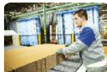
Corrugated board is cut to the required size before its final conversion into a box.
