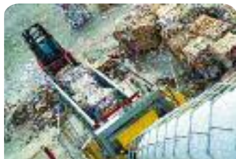
Bales of waste paper are taken into the new stock preparation plant at Kemsley Mill.
